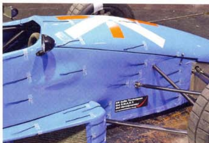
Upper centre wool tufts show the front suspension mounting brackets were disruptive
