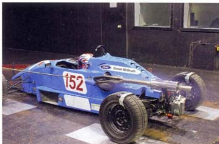
The exhaust headers and the regulation-spec silencer will also be adding unwanted drag
