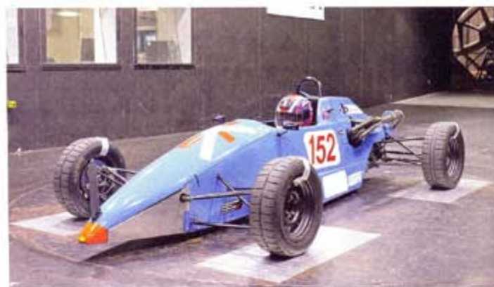
There is no downforce on the writer's Swift SC92F so the focus was on identifying drag sources. Note trip strips on tyres which simulate the flow separation on a rotating wheel
