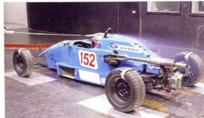
Flow down the rear of the engine cover was not fully attached; this could also add drag
