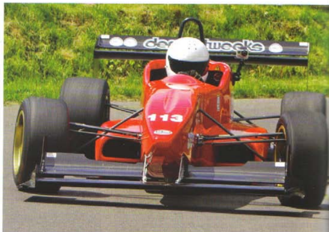
Where do you start with a front wing specification when there are few or no rules? This is the DJ Firehawk hillclimber, with a dual-element front wing
