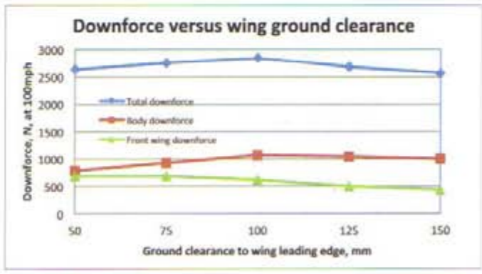
Figure 15: car body, front wing and total downforce vs wing ground clearance
