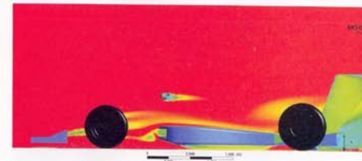
Figure 9: Total pressure losses caused by the mirrors were relatively short lived
