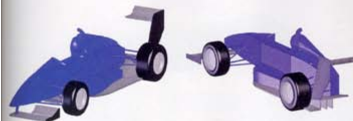
CAD 1: The single seater model used for our rear wing studies
