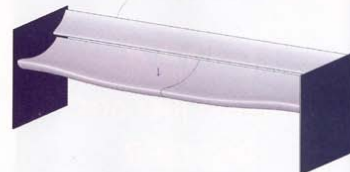
Figure 11: Rear wing Twist 1. Angle of attack at centre was increased by four degrees
