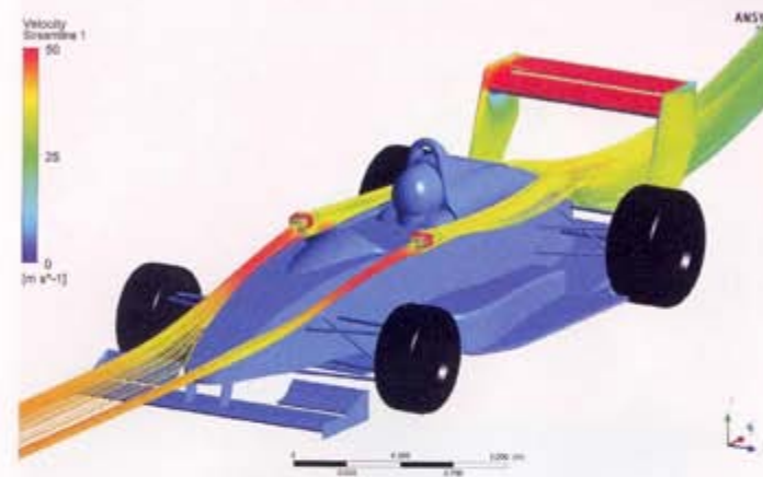
Figure 8: Surprisingly the mirror streamlines did not impinge on the rear wing
