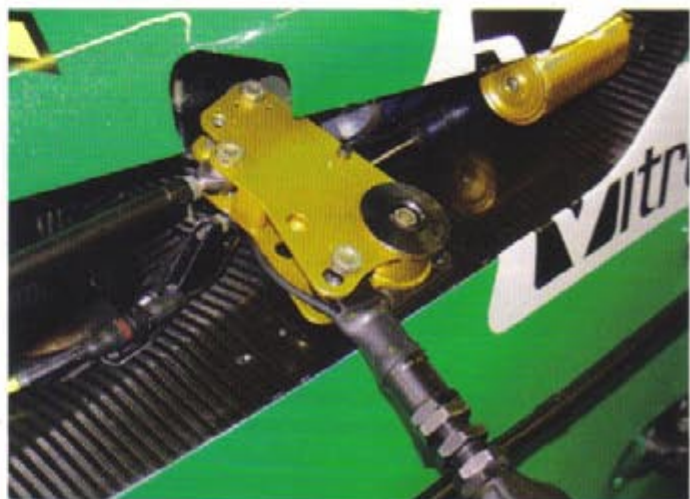
This 2002 Lola Champ Car was fitted with a strain gauge at the top of the pushrod (note the cable emerging from the insulation sheath, centre). A linear potentiometer can also be seen next to the damper body (centre top) (pic: T Webb)
