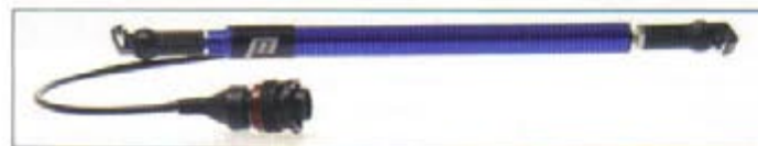
Above: a linear potentiometer rigged up to log suspension displacement on a Dallara F302 (pic: I McNeill). Below: a linear potentiometer (pic: P Rossard). Right: a linear potentiometer set up to log suspension displacement on a Honda Civic (pic: I McNeill)
